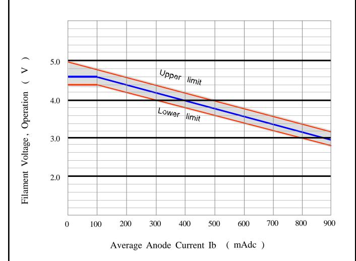
Fig. 1 Reduction Chart of Filament Voltage
