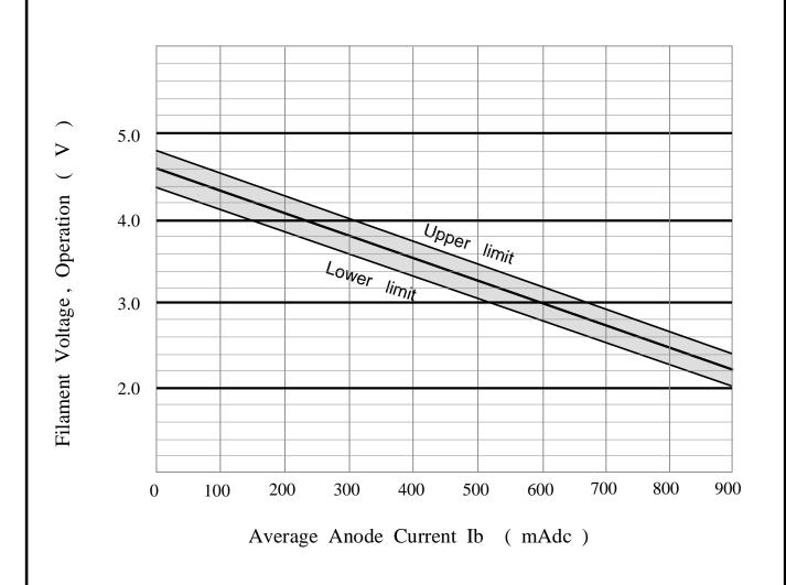
Fig . 1 Reduction Chart of Filament Voltage
